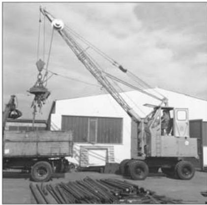
1962: Rope-driven S833 with elevated operator cab
