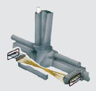
Cross controls Cross controls incorporate the same control lever sequence on either side of the truck, minimizing the risk of human error.
