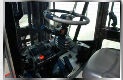
Spacious uncluttered cab with tilt steering, hinge-down dash, climate controls and adjustable seating Premium vinyl or cloth seat that rotates 15° left and 20° right
