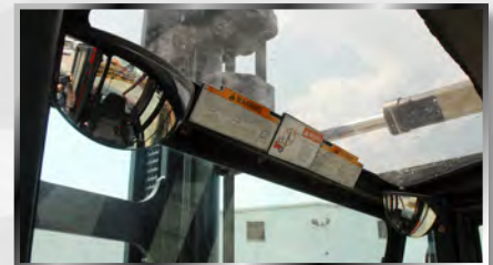
Dual panoramic interior rear view mirrors standard Dual external side view mirrors standard Optional pedestrian camera and monitor
