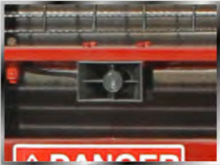
Reverse activated alarm Sloped counterweights for improved rear visibility
