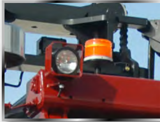
Overhead rear work lights for improved safety and visibility Key-switch actuated amber strobe light
