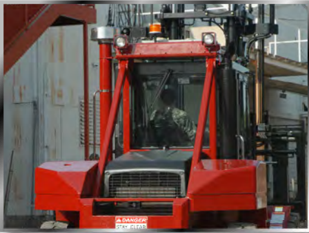
Unobstructed rear view The air snorkel and shielded exhaust are mounted on the corners of the cab to keep the view open.
