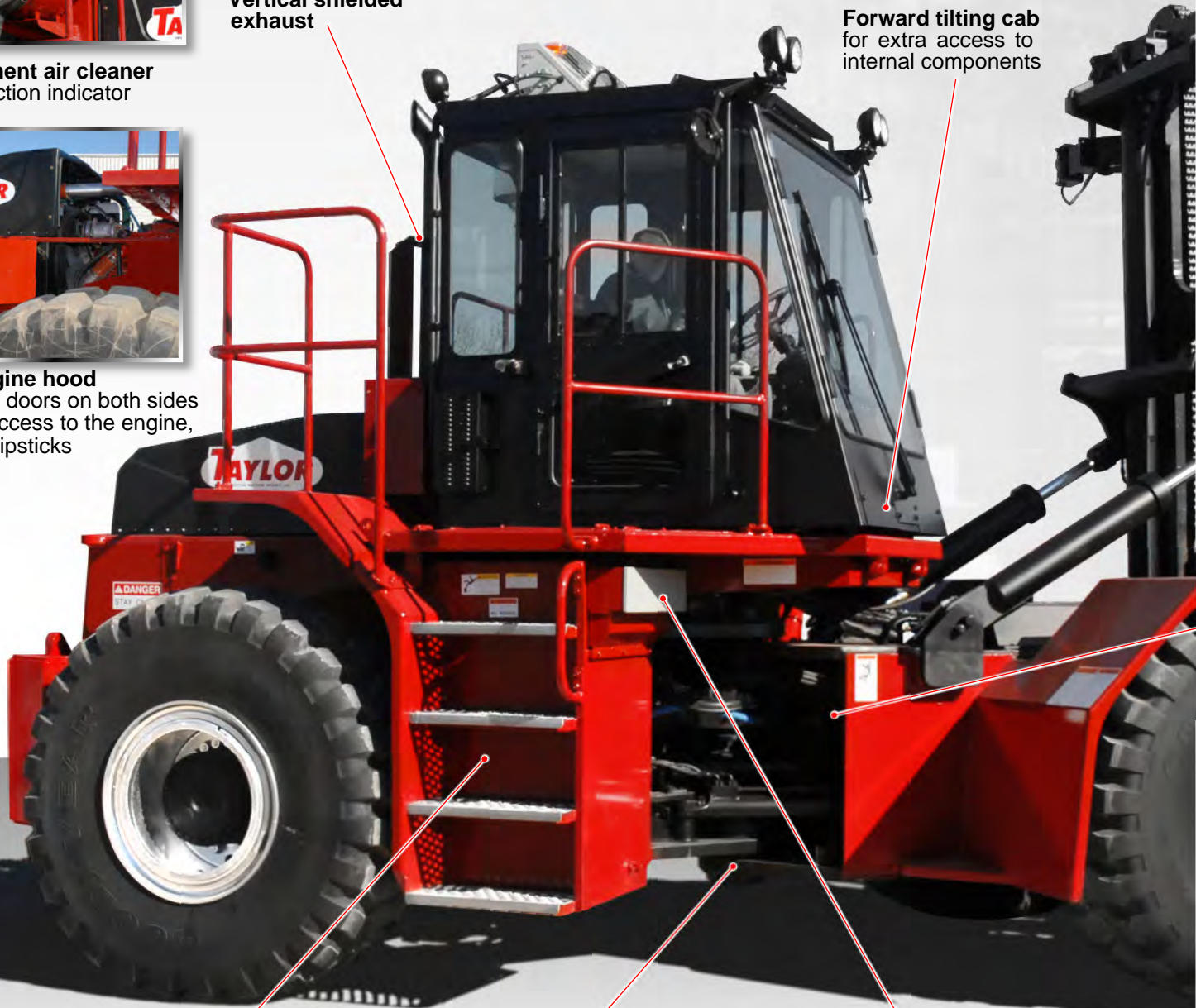
Hydraulic tank – • heavy gauge steel wall • serviceable filter element • tank mounted breather • internal suction screen • 55-gallon capacity Full flow, in-tank, 10-Micron return filtration
