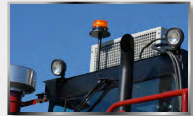
Overhead rear work lights for improved safety and visibility Key-switch actuated amber strobe light Reverse activated alarm
