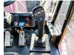
11 Button Command Joystick (Standard)
