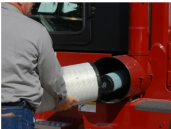
Donaldson Air Cleaner with Safety Element (Standard)
