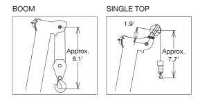
NOTE: Boom geometry shown is for unloaded condition and machine standing level on firm supporting surface.
