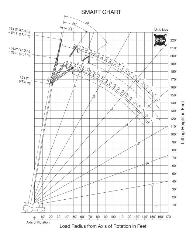
NOTE: Jib geometry shown is for unloaded condition and machine standing level on firm supporting surface.
