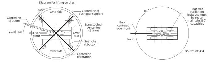
Bold lines determine the limiting position of any load for operation within working areas indicated.
