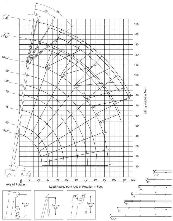
NOTE: Boom and jib geometry shown are for unloaded condition and machine standing level on firm supporting surface. Boom deflection and subsequent radius and boom angle change must be accounted for when applying load to hook.
