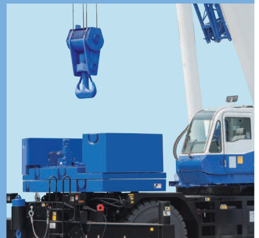
Counterweight mounting/dismounting cylinder
