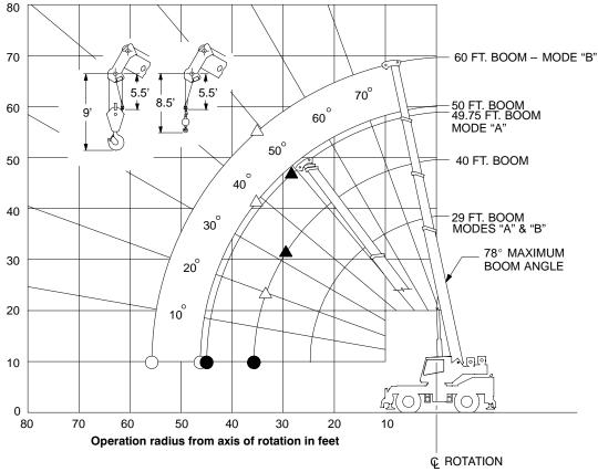
Crane Configurations Prohibited: Boom Lengths Greater than 60 FT. 25 Ft. Fixed Fly 27 Ft. Offset Fly 44 Ft. Offset Fly
