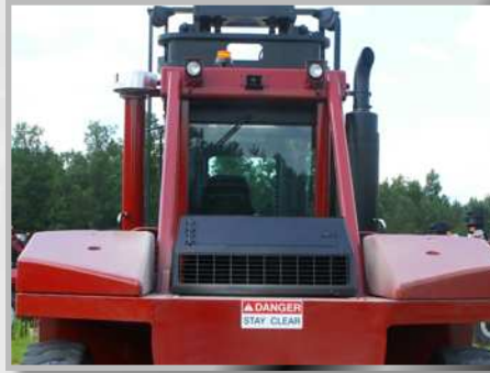
Unobstructed rear view The air snorkel and shielded exhaust are mounted on the corners of the cab to keep the view open.
