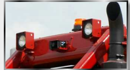
Overhead rear work lights for improved safety and visibility Key-switch actuated amber strobe light Reverse activated alarm
