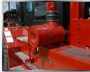
Dual element air cleaner with restriction indicator
