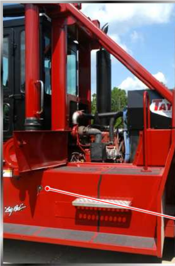
Battery cut-off switch
