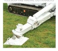
PRESSURE SENSING, SWIVEL FOOT ALLOWS EASY SET-UP
