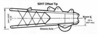
The 92HT boom is suspended by four part pendants from the outer bail to the boom tip. Pin connected center sections with matching pendants are available in 10 ft. (3 m), 20 ft. (6.1 m) and 50 ft. (15.2 m) lengths.
