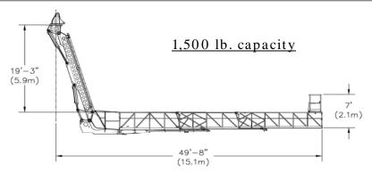
The Aspen A-52 can be equipped with an interchangeable work platform. This 43' long steel walkway can extend close to 50' horizontally under the bridge. It is kept level by means of a hydraulic leveling system and comes equipped with a "step up" platform for access behind deep girders. Wireless controls enable the workers to move the unit from anywhere along the platform.
