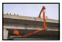
Two platform options are available. Either a telescoping boom with an articulating 4th boom and inspection platform, or a 1,500 lb 3-stage walkway can be installed.
