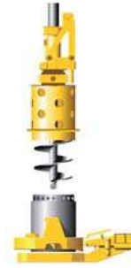
Cased Kelly Drilling (installation with oscillator)
