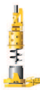
Cased Kelly drilling (installation with oscillator)
