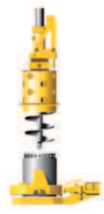
Cased Kelly drilling (installation with oscillator)
