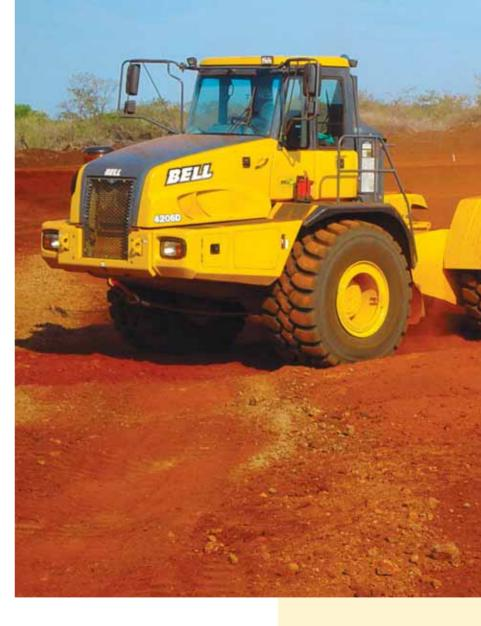
• Gross Power : 205 kW (275 hp) • Gross Torque : 1 000 Nm (736 lbft) • Gross Weight : 12 120 kg (26,712 lbs)
