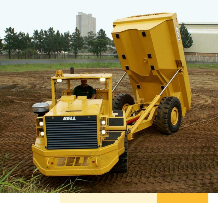
Gross Power: 205 kW (275 hp) Gross Torque: 1 100 Nm (850 lbft) Rated Payload: 27 000 kg (59 524 lbs)
