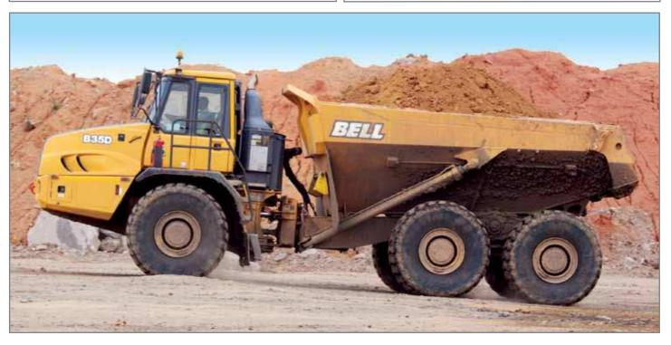
• The exclusive onboard weighing option presents the operator with real time information on the payload while the machine is being loaded. A 'limp home' mode can also be activated if the machine is significantly over-loaded.
