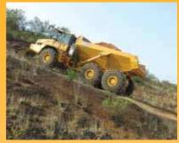
• The incorporation of a Pitch and Roll sensor in the vehicle allows the bin to not be operated if the truck is in an unsafe position.
