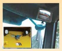
Optional Tyre pressure - monitoring System ensures that the operator has real time information on all tyres pressure and temperature conditions.
