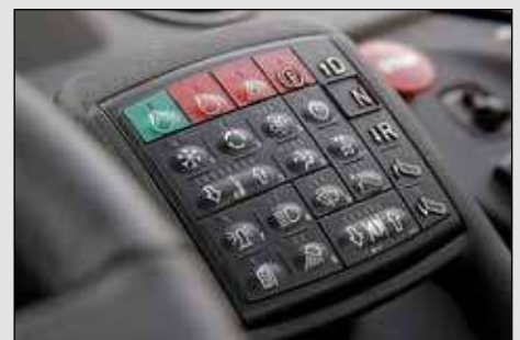
Keyless start, driver identity and access codes ensure no unauthorized operation of your equipment.
