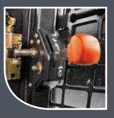
**Convenient engine speed control:** The engine speed control is in front of the operator, on the right-hand corner post of the cab. Easy to reach and to control.
