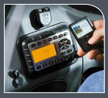
Radio-ready and 12-Volt power accessory: All our loaders can be easily equipped with a stereo radio. The radio features an auxiliary audio input jack that is ready for an MP3 player or similar devices. And, because your cab is your office, we've installed a 12-Volt power accessory for charging your mobile phone, MP3 player or other accessories.
