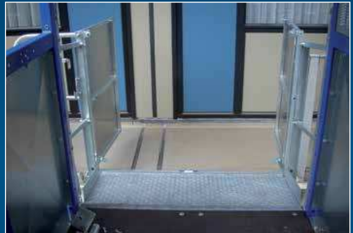
Landing with opened platform ramp
