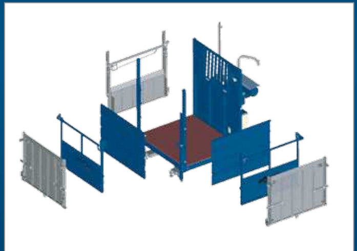
Possible base-unit extensions with gates, ramps and closing walls
