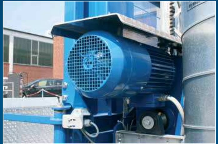
Powerful drive units ensure high lifting speeds up to 131 ft/min / 40 m
