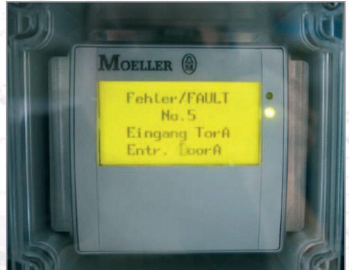
Errors are automatically shown on the display (optional)
