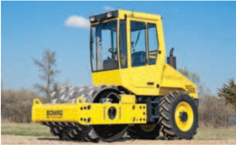
Optional cab provides all weather protection.
