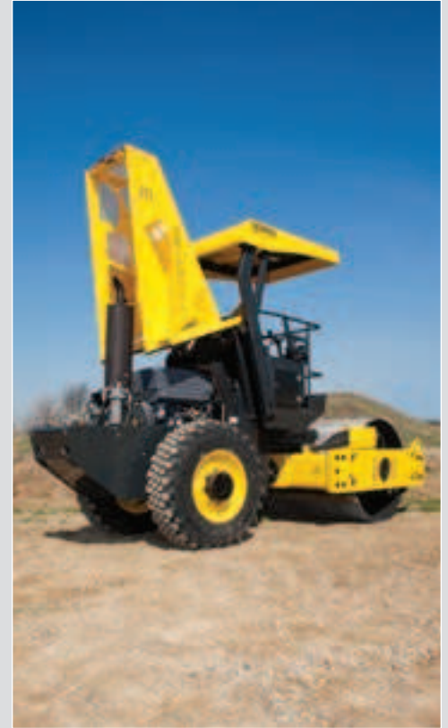
Wide opening hood provides easy access to all components.
