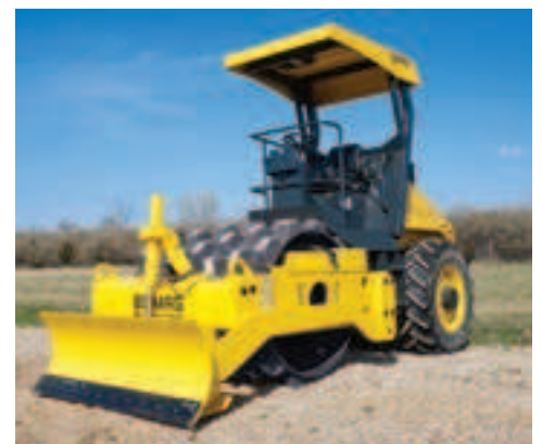
BW145PDH-40 Padfoot model for cohesive material applications. Also available with optional leveling blade.
