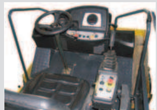
Ergonomic layout of operators platform and controls.
