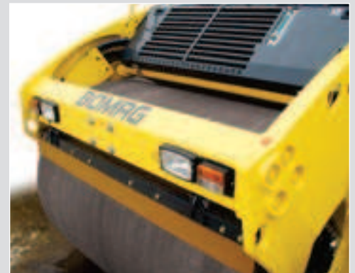
Two spring loaded scrapers per drum allow easy cleaning and replacement.
