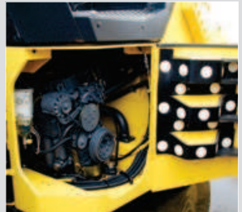
Easy access to engine and hydraulic components from either side.
