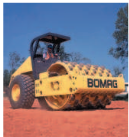
Designed specifically for soil compaction.
