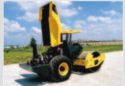
Vertically Opening Hood for Maximum Serviceability
