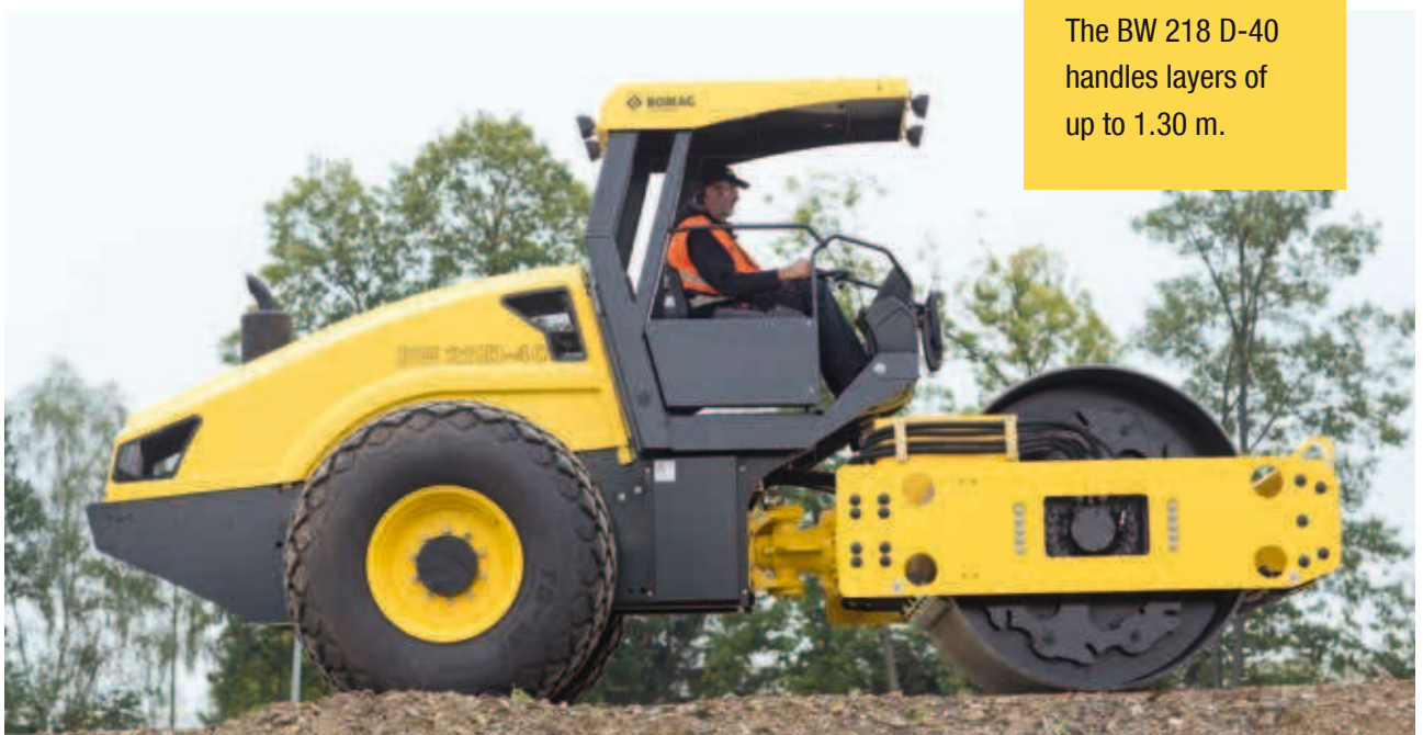
Power and endurance: Vibration with high amplitudes, encased bearing and internal cooling.
