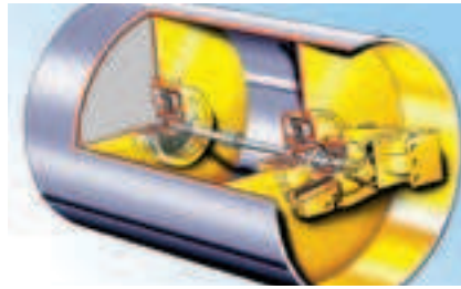
Standard dual amplitude and frequency enhances machines versatility
