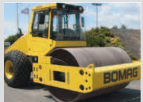
Optional ROPS cabin with available heating and air conditioning.
