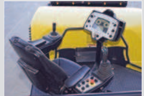
Joystick control travel direction, speed, steering, manual vibration on/off and control actuation from either seating position.
