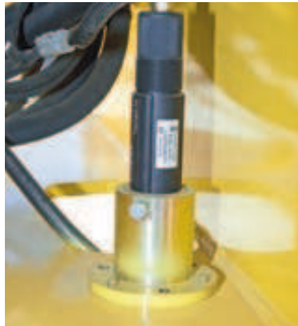
The optional Asphalt Mat Temperature Sensing System measures the material temperature which is critical for asphalt mix projects.
