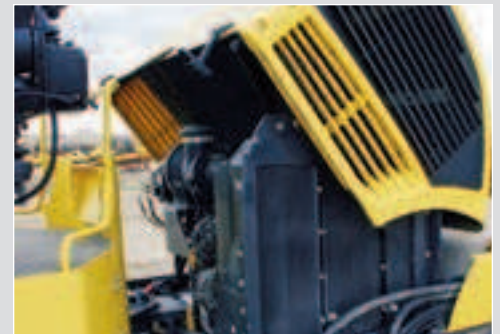
Vertical side by side coolers allow easy access for quick cleaning.
