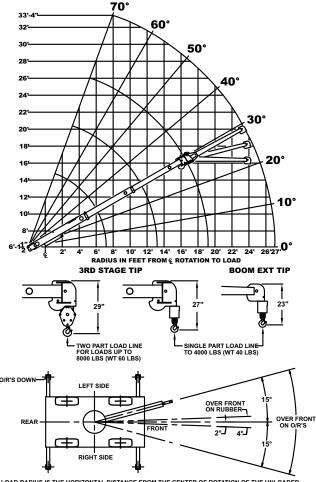
LOAD RADIUS IS THE HORIZONTAL DISTANCE FROM THE CENTER OF ROTATION OF THE UNLOADED CRANE TO THE VERTICAL LOAD LINE WITH THE LOAD APPLIED.
