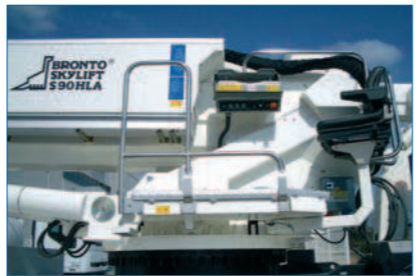
Full turntable control station with seat, identical to the working cage control station.
