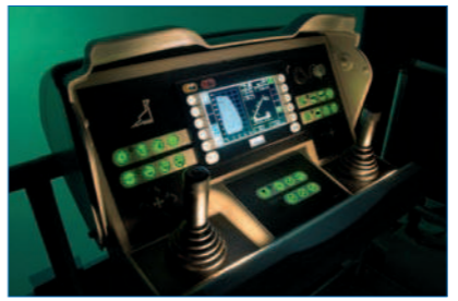
All HLA units have Bronto+ electronic control system including geometry based outreach control system, giving exactly identical outreach under all circumstances.
