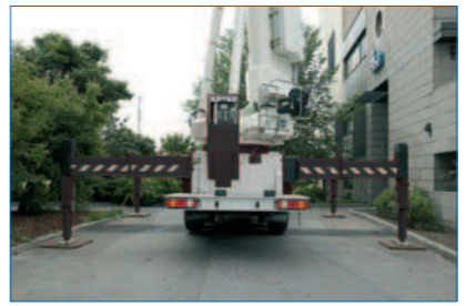
With the easy automatic levelling function the unit is fully stabilized in 40 seconds. Returning of the outriggers into transport position is automatic by one push-button.
