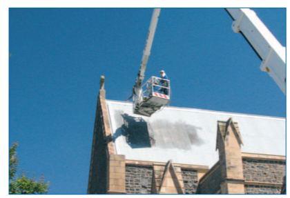
Cage slewing 90 degrees. Hydraulically extendable cage available as an option.
