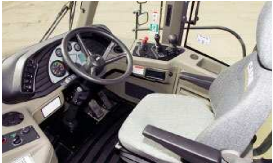
The right-hand console is designed to provide better operator control. Among its operator-friendly features are: push-button change from manual to automatic shift and bump shifting.
