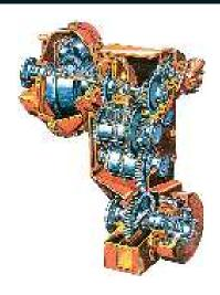
An electronically-controlled transmission provides the operator with a choice of fully automatic operation or manual powershift control. Six forward ratios and three reverses gears enable full use of the engine power in all ground conditions. Precise clutch engagement and smooth gearshift modulation result in extended driveline component life and reduced fatigue for the operator.
