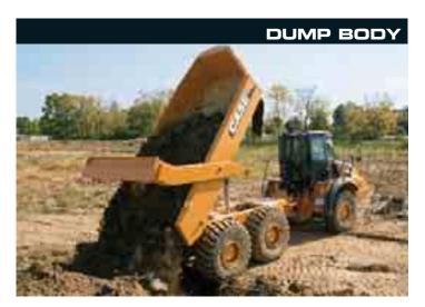
The Case B series articulated truck has a wide chassis and dump body to provide a lower centre of gravity, increasing stability on rough ground and assisting the suspensions system to provide a smooth ride. The tilt cylinders are mounted within the wide frame rails, for added protection and to improve the lift geometry for rapid discharge and return to hauling position.
