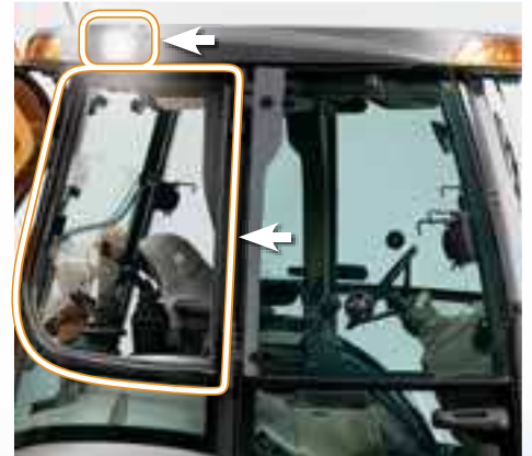
New rear-quarter windows and side lighting
