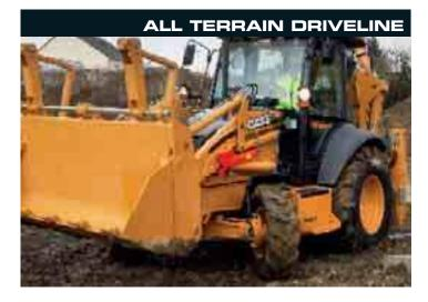
The 580 Super R Series 3 and 590 Super R Series 3 are all weather, all terrain machines, their four wheel drive providing traction in the worst site conditions. Customers can choose between the robust design of a mechanical PowerShuttle transmission, offering four forward and four reverse gears, or the smooth shifting PowerShift transmission that has four forward and two reverse speeds.
