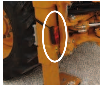
Rear road lights can be fitted on the stabilizer legs while traveling and on the cab when digging, providing maximum visibility and protection
