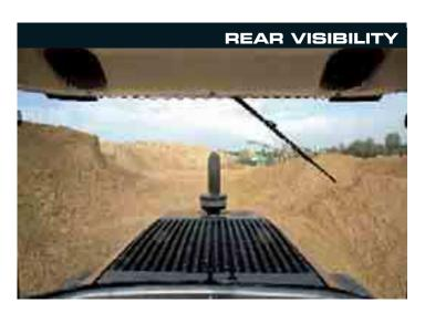
At the rear of the machines a contoured one-piece engine canopy drops away from the line of sight to give an excellent view behind the operator. The engine air pre-cleaner and exhaust stack are positioned in line in the centre of the canopy to further increase visibility over the back of the machine.
