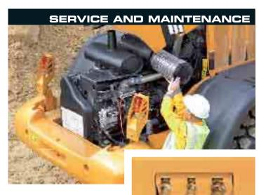
With the mid-mounted cooling module, the engine sits right at the rear of the machine, beneath a single-piece electrically-operated engine cover. The engine therefore contributes to the machine counterweight, reducing the need for additional counterweight at the rear
