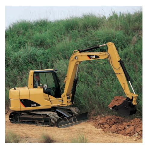
**Linkage Bearings.** New bearing technology has extended the front linkage greasing intervals for all bearings except the bucket.
