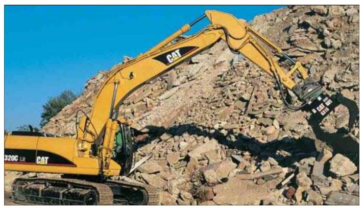
**Booms and Sticks.** Built for performance and long service life, Caterpillar booms and sticks are large, welded, box-section structures with thick, multi-plate fabrications in high-stress areas.
