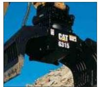
**Multi-Processor.** The Caterpillar Multi-Processors can be equipped with different jaw types depending on your need.
