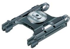
**Undercarriage.** Durable Cat undercarriage absorbs stresses and provides excellent stability.
