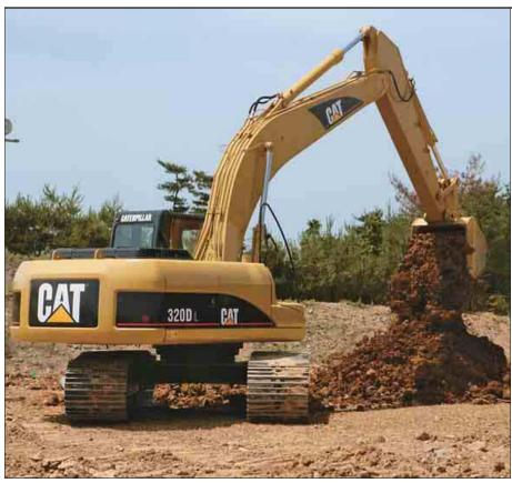
**3066 ATAAC Engine.** The Cat 3066 is a six-cylinder turbocharged and aftercooled engine. The engine features long-stroke piston movement for high torque at medium to low speeds, which provides excellent productivity in the toughest working environments. With the new Economy Mode, customers can balance the demands of performance and fuel economy to suit their requirements and application.
