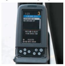
**Monitor.** The monitor is a full color 400x234 pixels Liquid Crystal Display (LCD) graphic display. The monitor angle can be adjusted to minimize sun glare and has the capability of displaying information in Indonesian and twenty-six other languages.
