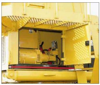
**20 kW hydraulically driven generator set** can power magnets up to 1702 mm (67") in diameter. A Baldor generator and a state-of-the-art electronic magnet controller, manufactured for Cat by Crane Systems Inc., are linked to provide trouble free service. This new controller completely eliminates traditional contactor maintenance and it is supported and warranted through your Cat dealer.
