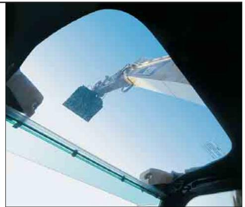
**Skylight.** A unique large polycarbonate skylight provides very good upward visibility, especially useful in above ground applications.
