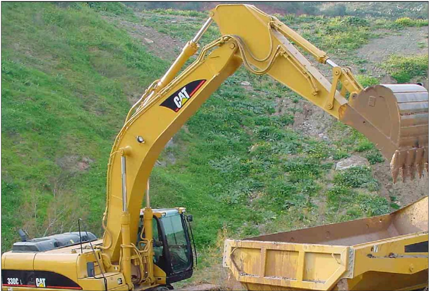
**Booms and Sticks.** Built for performance and long service life, Caterpillar booms and sticks are large, welded, box-section structures with thick, multi-plate fabrications in high-stress areas.
