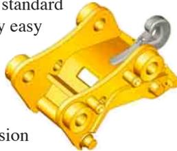
**Pin Grabber Plus Quick Coupler.** This hydraulically controlled Pin Grabber Plus quick coupler makes changing buckets and other popular work tools simple and fast. The Pin Grabber Plus coupler mounts to the end of the stick and allows buckets, clamshells and other work tools to be used with little or no modification.
