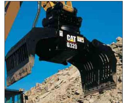
**Multi-Processor.** The Caterpillar Multi-Processors can be equipped with different jaw types depending on your need.
