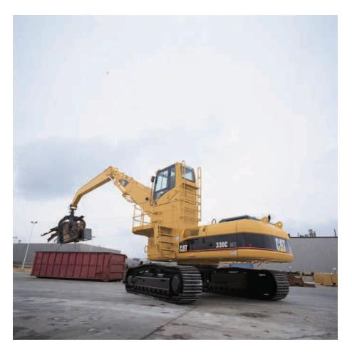
**Engine.** Six-cylinder, turbocharged engine built for power, reliability, and economy will allow the machine to consistently perform at high levels. The Cat C9 engine is designed for low emissions and will meet EPA Tier 2 and EU Stage II emissions requirements.
