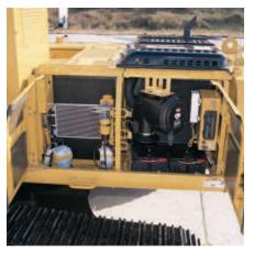
**Side-By-Side Cooling System.**The C-Series side-by-side cooling system is separated to prevent stacking of debris and allow easier access for cleaning.
