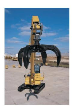
**Cat Orange Peel Grapples.** The 1.25 CYD (0.96 cu. m) Orange Peel Grapple is constructed with four wear-resistant steel tines and fully replaceable tips for excellent service life.
