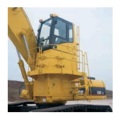
**Cab Riser.** Cat designed and built, 77" (1.95 m) manual tilt cab riser provides for operating height with excellent visibility for loading and unloading processing equipment, trucks, and rail cars. Access to the cab is provided by a ladder to the platform extending around the cab riser. This platform allows windshield cleaning. The cab riser can be manually tilted forward 90 degrees for shipping.
