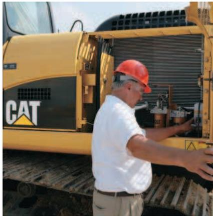
**Radiator Compartment.** The left rear service door allows easy access to the engine radiator, oil cooler and air-to-air-after-cooler. A reserve tank and drain cock are attached to the radiator for simplified maintenance.
