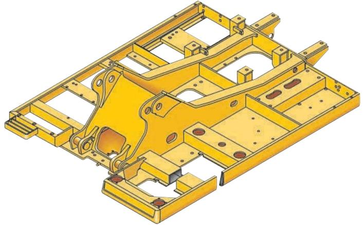
**Robotic Welding.** Up to 95% of the structural welds on a Caterpillar® Excavator are completed by robots. Robotic welds achieve over three times the penetration of manual welds.
