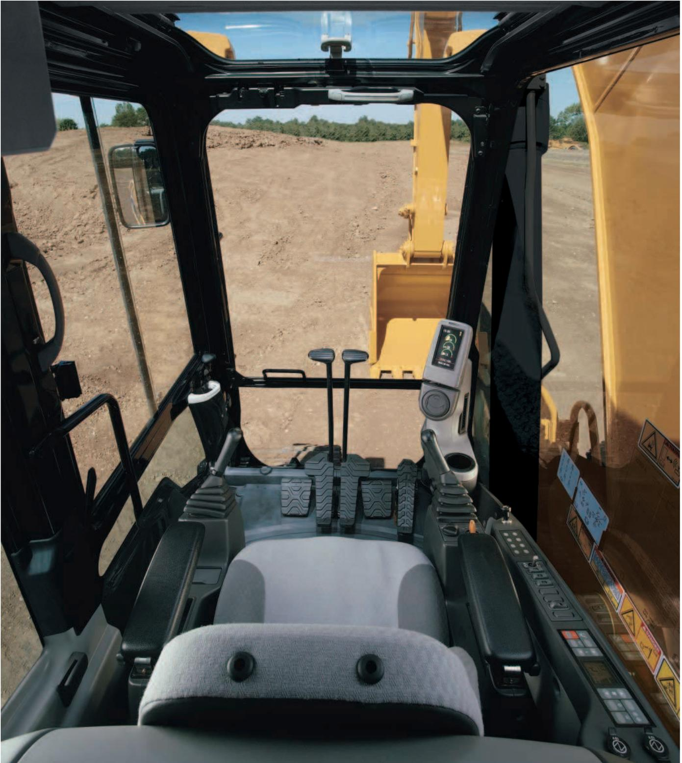
**Operator Station.** The workstation is spacious, quiet and comfortable, assuring high productivity during a long work day. The air conditioner and attachment switches are conveniently located on the right-hand wall, and the key switch and throttle dial are on the right-hand console. The monitor is easy to see and maximizes visibility.
